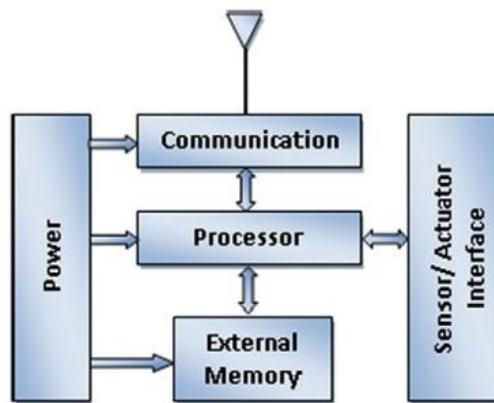
Fig (2): Architecture of WSN node
